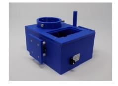
The EvoluChem™ PhotoRedOx Box is equipped with several mirrors that direct and distribute the light toward the sam-ples. The geometry of the box enable par-allel reaction with homogenous light ex-posure.
